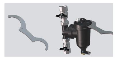
To inspect the desludger completely or clean/replace the filter cartridge, you can remove the top cap completely with the provided wrench.
