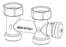
The by-pass for the primary circuit (optional) allows the hydraulic separation between the primary and secondary circuit. This hydraulic separation optimizes the operation of the secondary circuit and prevents changes in the flow rate of the primary from affecting the secondary circuit. The flow rate that passes through the respective circuits depends exclusively on the flow rate characteristics of the pumps, avoiding the mutual influence due to their coupling in series.
