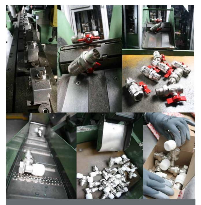
ITAP can count on 55 automatic assembly and testing lines; every day about 400,000 valves are fully assembled, tested and delivered to the storage warehouse and made ready for dispatch.
